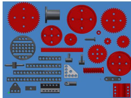
Figure 15: Inventa parts give strength, precision and connectivity to junk and recycled materials used in maker tasks. They speed up construction time: an important feature in a busy classroom schedule. Making them freely available for 3D printing will make them low-cost and improve the success of maker projects.
