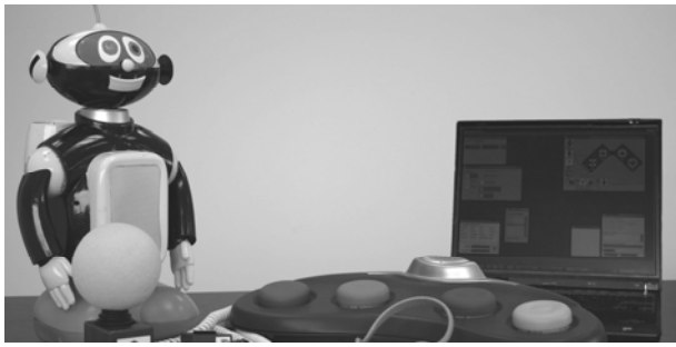
Fig. 1. CosmoBot™ Learning System with graphical user interface and robot for therapy, education and play.
