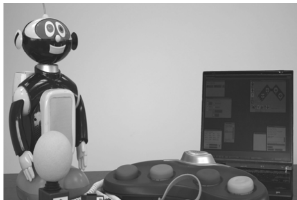
Fig. 1. CosmoBot™ Learning System with graphical user interface and robot for therapy, education and play.
