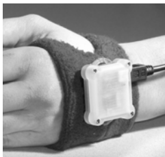
Fig. 3. Three degree-of-freedom accelerometer enclosed in sealed case and attached on dorsum of hand.
